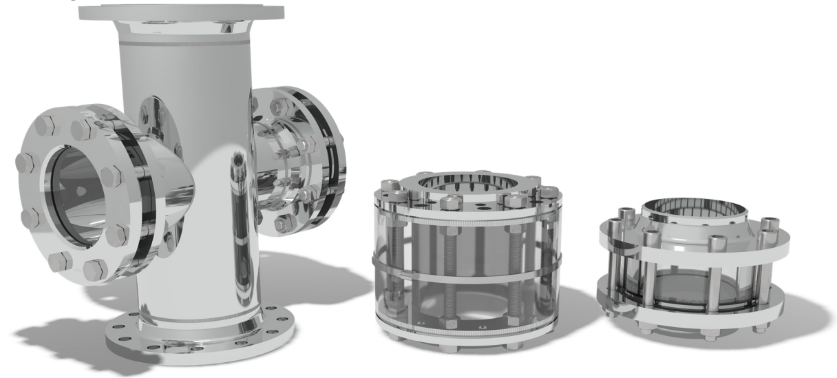
Figure 5: Typical flow sight glasses. From left to right: Welded body with flange connections, tubular sight glass with impact protection shell, intermediate flange sight glass (here installed between two welded neck flanges).
