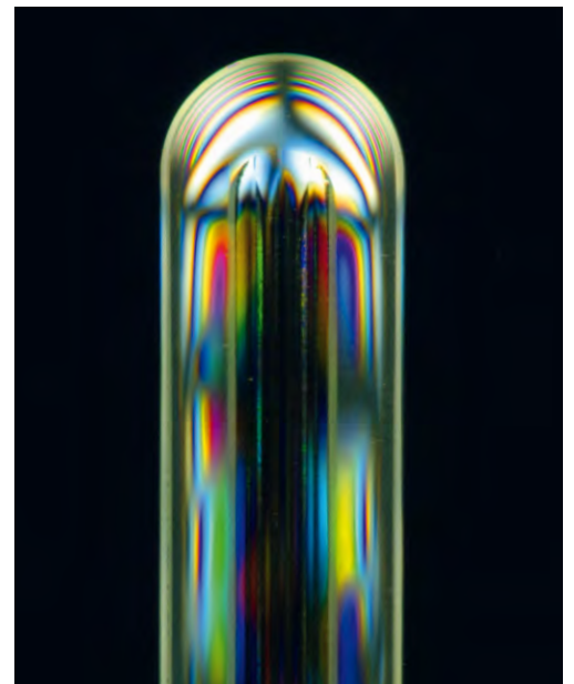
Special tempered MAXOS® glass under polarized light.
